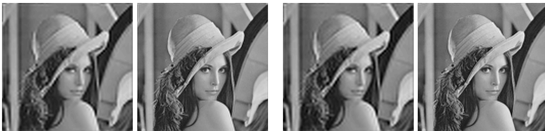
Figure 7.15: M1 Coiflet 17-11: LL: b/p = 0.35 PSNR=26.61, L: b/p = 1.40 PSNR=30.65, Optimized 17-11: R: b/p = 0.33 PSNR=26.70, RR: b/p = 1.35 PSNR=30.74
