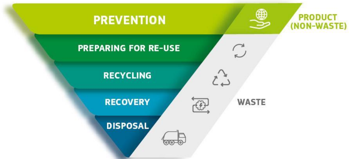
Figure 8: Depiction of the waste hierarchy as set by the EU. Source: European Commission (2022)
