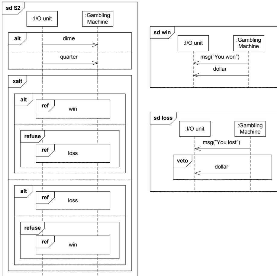
**Fig. 3.** Sequence diagram with inherent nondeterminism (xalt)
