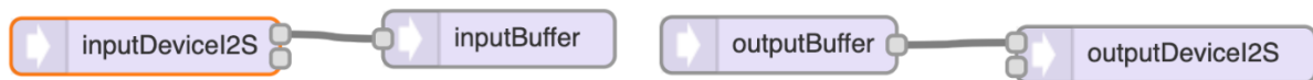
Figure 4.3.1 Teensy Audio GUI Representation of the Audio Data Routing for the Buffer Passthrough Test
