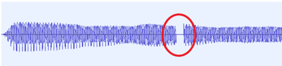
Figure 5.1: Audio dropout. The red circumference points out an interruption in the audio signal, which can be translated in an unpleasant cracking sound through loudspeakers.
