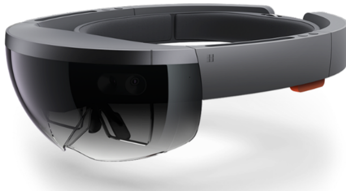
Figure 4.20: Microsoft HoloLens (Version 1). A high-precision mixed reality headset.
