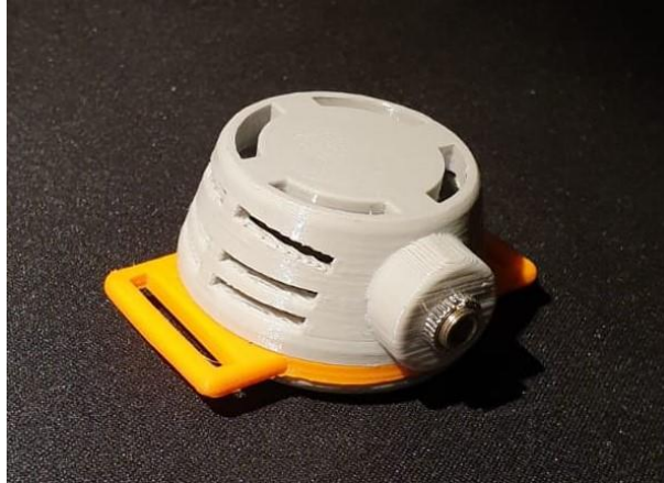
Figure 3.1.1 The hap-phones, created after based on the design proposed by Yao and Hayward (2010)
