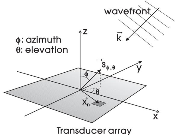
Figure 1. A 2D planar array with coordinate system.
