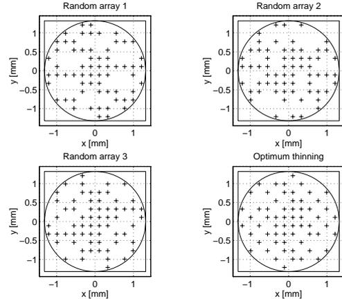
Figure 3. Element layouts for 112 element full array thinned to three different random 64 element layouts and a 62 element optimized layout. The random arrays are sorted according to the peak sidelobe level in Fig. 2 with Random 1 having the highest peak sidelobe level for large beamwidths.
