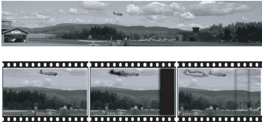
Figure 3.1: Three frames from a video where the camera follows the airplane, panning to the right. The dark eras in frame two can be reconstructed from the outlined eras in frame three, but are not present in frame one.
