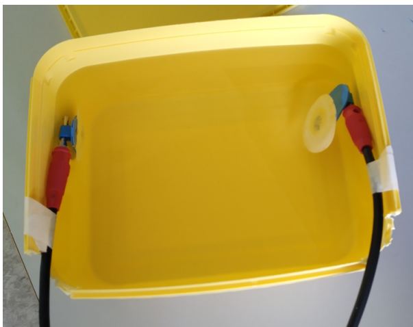
Figure 3.1: The Reference ECG electrode and the Counter ECG electrode in the plastic tank with saline.
