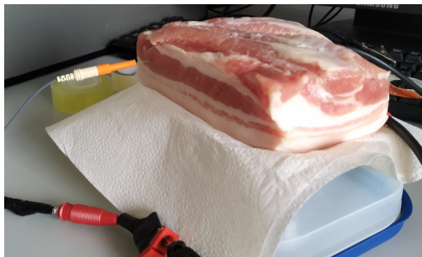
Figure 3.4: The needle positioned in muscle tissue in a piece of side meat. The needle is of type 1 (Teca). The two ECG electrodes are positioned on the skin underneath and out of sight at the back of the side meat.
