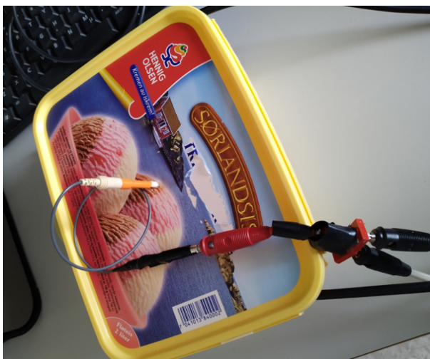
Figure 3.2: The needle is supported by a plastic tube, with a small diameter, through the lid of the tank with saline. The needle is of type 1 (Teca).
