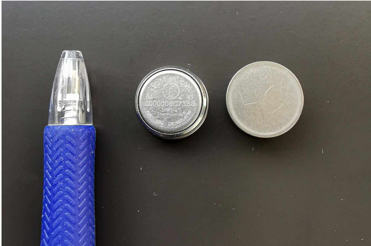
Figure 3. iButton temperature sensors used for measuring skin temperature in Study II. (Photo by Jørgen Melau)
