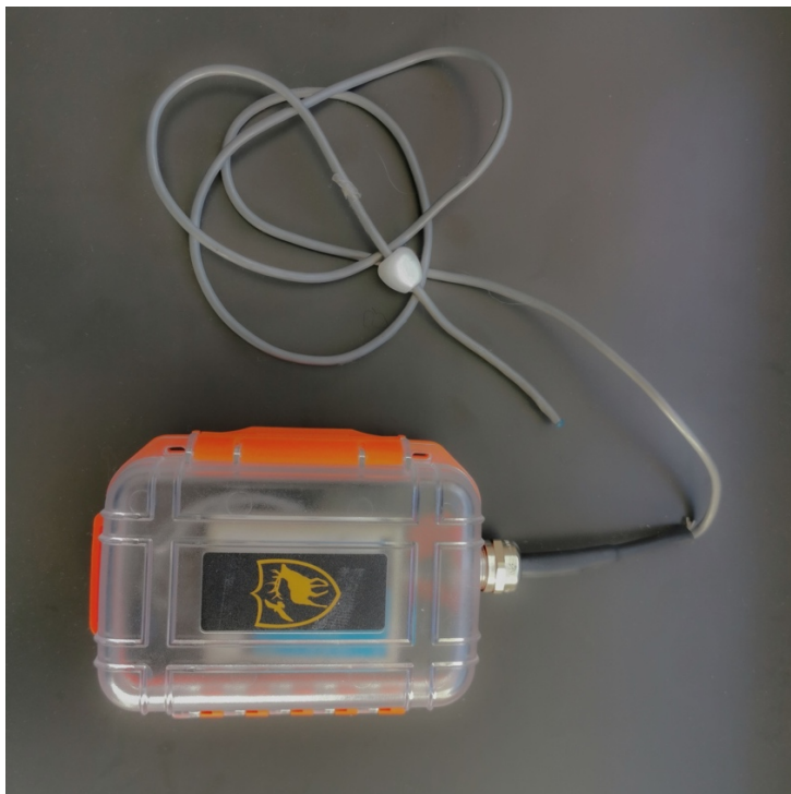
Figure 1. The wired rectal probe and the watertight box for the logger used in Study I. (Photo by Jørgen Melau)
