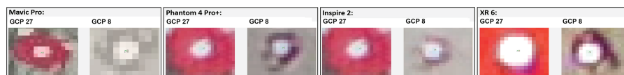
FIGURE 7 Different image resolution covering selected GCPs in the UAS datasets. Ground-sensor distances are 50 m (GCP 27) and 80 m (GCP 8) [Color figure can be viewed at wileyonlinelibrary.com]
