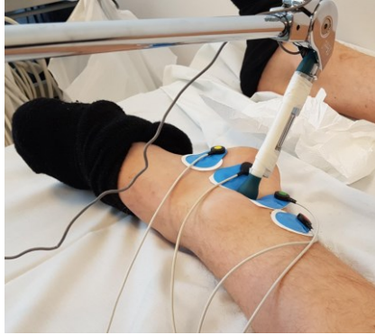
Figure 1: Illustration of posterior tibial artery with the tonometer between the four electrodes.
