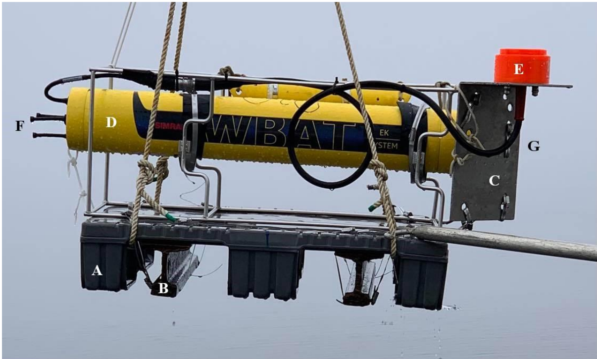
Figure 9: The echosounder as deployed. The letters illustrate the different components assembled to construct Simrad WBAT echosounder rig: A) Plastic pallet B) Train tracks C) Steel frame D) Transceiver E) Transducer F) Transducer end cap G) Communication end cap.
