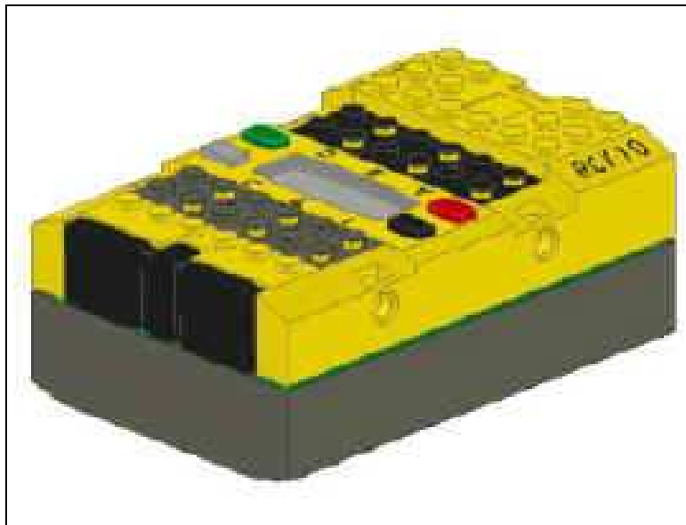
Figure 3.1: The heart of the Lego Mindstorms robot. The RCX
