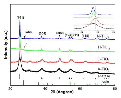
Figure 2. XRD patterns of the prepared TiO<sub>2</sub> nanocrystals.
