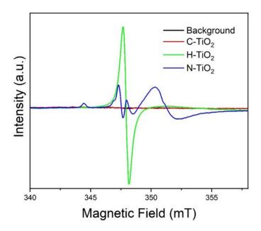
**Figure 6.** EPR spectra of paramagnetic species in C-TiO<sub>2</sub>, H-TiO<sub>2</sub> and N-TiO<sub>2</sub>. Spectra in this display have not been adjusted for slightly different microwave frequencies or for slightly different sample weights. The frequencies were 9755.2 MHz, 9755.0 MHz, 9753.3 MHz and 9754.3 MHz for background, C-TiO<sub>2</sub>, H-TiO<sub>2</sub> and N-TiO<sub>2</sub>, respectively.
