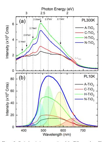
**Figure 5.** Optical emission properties of the  $TiO_2$  powders: PL spectra measured in vacuum at 300 K (a) and 10 K (b). The key emission components are indicated by Gaussian deconvolution curves/shaded areas.
