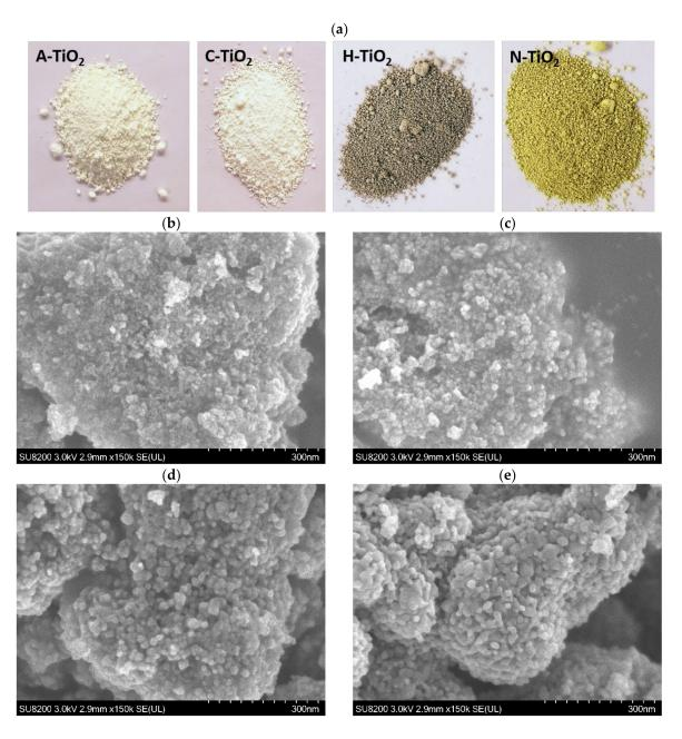
**Figure 1.** Photographs of the investigated TiO<sub>2</sub> nanocrystals (**a**) and representative SEM images of A-TiO<sub>2</sub> (**b**), C-TiO<sub>2</sub> (**c**), H-TiO<sub>2</sub> (**d**), and N-TiO<sub>2</sub> (**e**), respectively. Scale bar: 300 nm.
