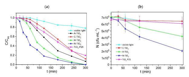
**Figure 7.** Photocatalytic decolorization of MG (**a**) and inactivation of *G. stearothermophilus* endospores (**b**) under visible light illumination. In all cases  $0.5 \text{ g L}^{-1}$  of the corresponding photocatalyst were used.
