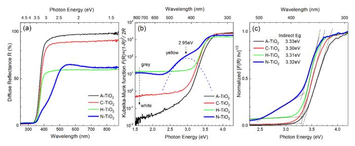
**Figure 4.** Optical absorption properties of the  $TiO_2$  powders: diffuse reflectance (**a**), modified Kubelka-Munk function (**b**), Tauc plot assuming indirect (allowed) transitions (**c**).
