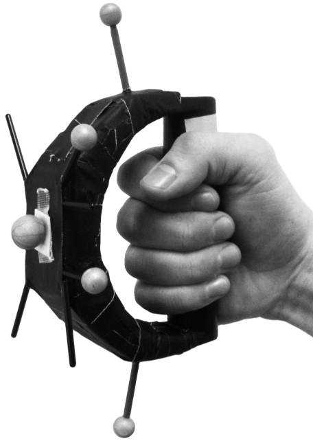
Fig. 1. One of the two handles that was used for recording the participant's motion.
