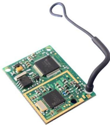
**Figure 2: The Tinynode sensor node. Image from [8]**
