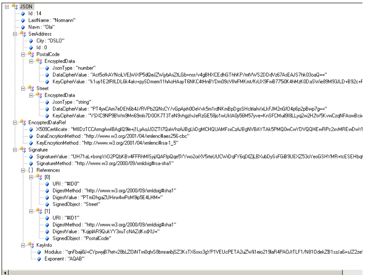
Figure 5.11: A compressed JSON message with encrypted and signed Street and PostalCode -elements, shown in JSON Viewer
