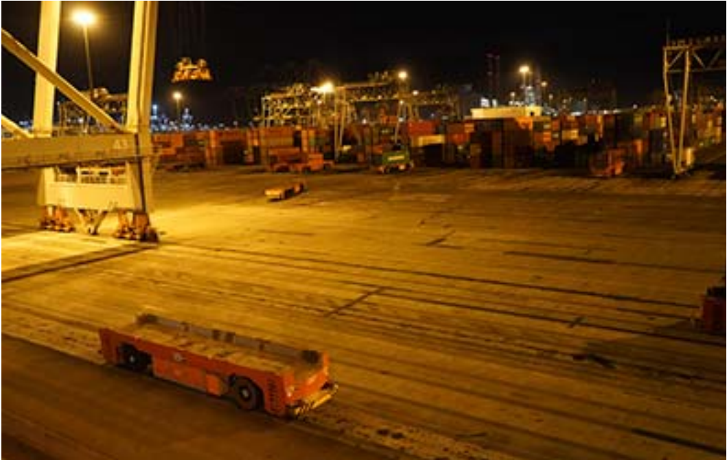
FIGURE 3. Driverless trucks in one of Rotterdam's container terminals. Photo by Johanna Markkula.
