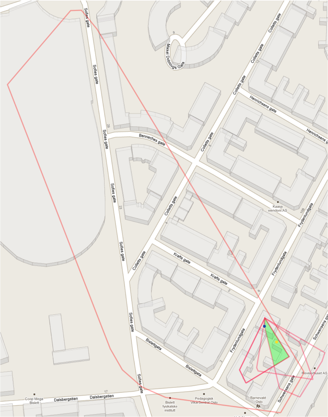
Figure 4.7: Live example of the Intersecting Areas location estimation method. The intersection of the red areas are found to produce the green estimated location area. The yellow point is the estimated location and the blue point is the true location.
