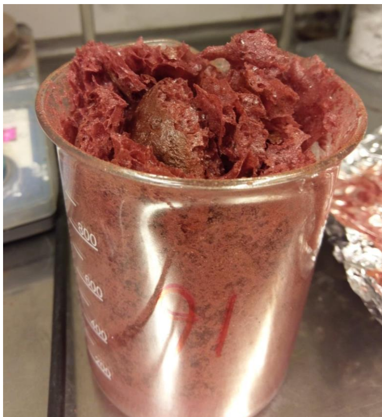
Figure 10 – Xerogel for BGLC synthesis after drying the mixed precursors at 250 °C.
