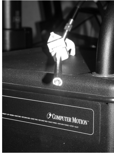
Figure 7.7: As can be seen as a glowing ring on the endoscope the light will be elliptically shaped in the images. Viewing an object at close range yields images where the light do not cover the entire image thus giving images with uneven lighting. This can clearly be seen in figure 7.5.
