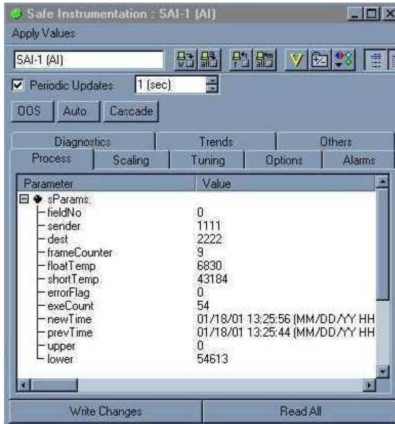
Figure 6-1, The block window. This window displays a function block's parameters as they appear in the block or you can choose which of the parameters you want to display. In this figure only the safetyParams-struct in the SAI-1 is block shown. The SAI-1 is here sending the first field of the tenth frame.
