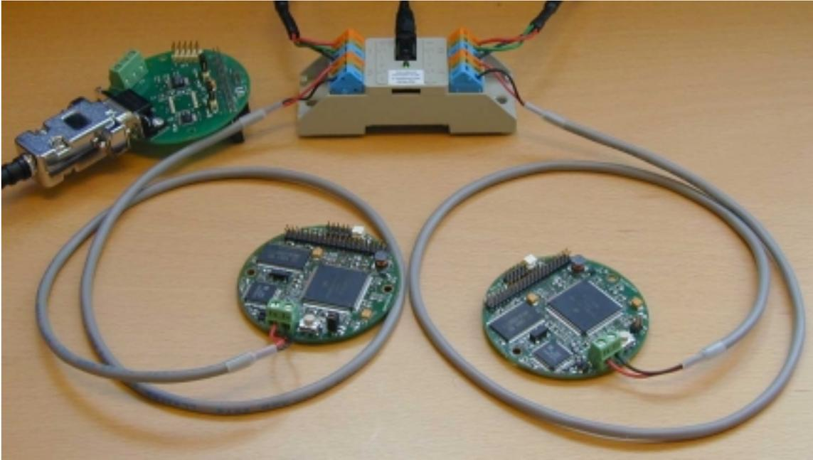
Figure 2-7, The picture shows the Fieldbus “Power hub,” two development round cards in the foreground and the serial programming daughter card is up in the left corner.
