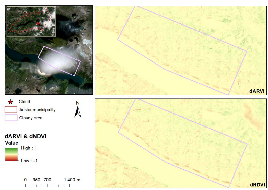
Figure 18: dARVI and dNDVI calculated with Landsat 8 data displayed over the cloud-affected area in Sentinel 2A.
