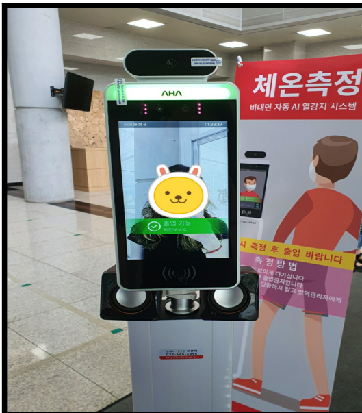
Figure 6: AI device that checks your temperature and whether you are wearing a mask or not
