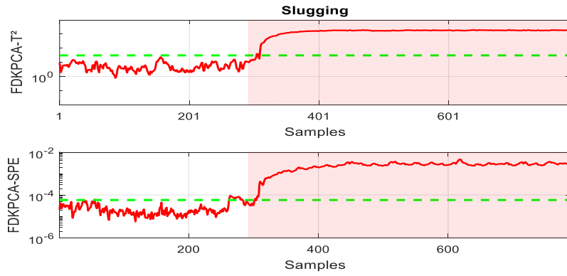
Fig. 8. Monitoring results of FDKPCA model using T^2 and SPE at 99% CL of slugging condition
