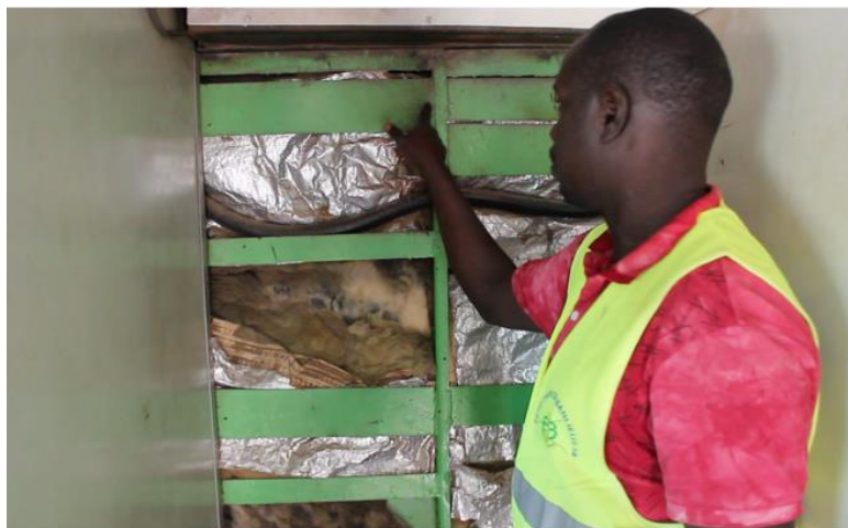
Fig. 4 Abdoulaye explaining the insulation system of a train
