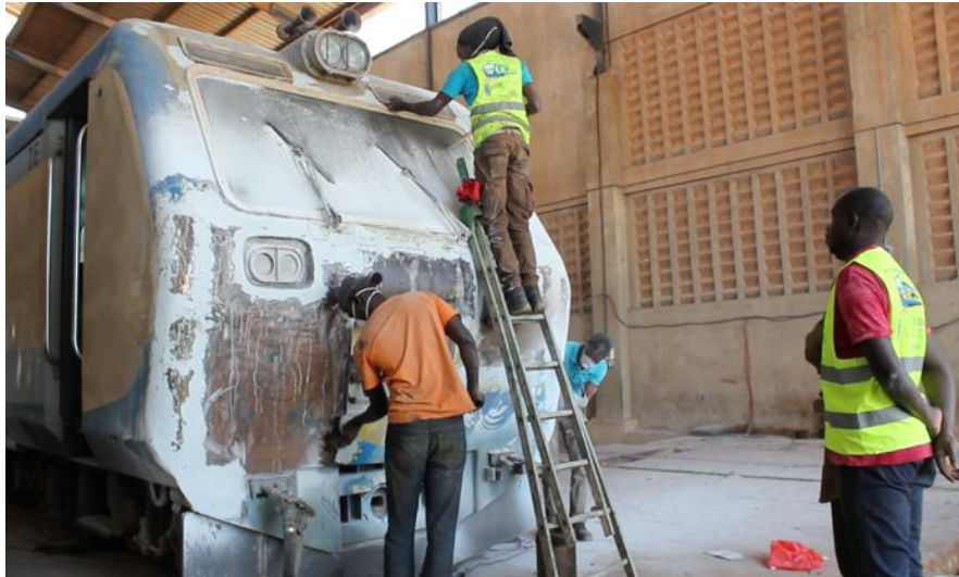
Fig 8. Workers sanding a locomotive before applying paint in the depot of Rufisque
