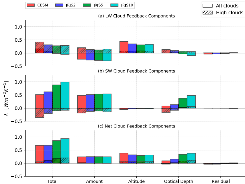
FIG. 9. Global mean cloud feedback contributions separated into cloud-amount, cloud-altitude, and cloud-optical-depth components computed from cloud fraction histograms with cloud-optical-depth and cloud-top-pressure bins. A separate decomposition is performed for high clouds (<440 hPa), shown with hatched bars. Note that these high-cloud components are only useful for magnitude comparison because they are not additive with low-cloud (i.e., >440 hPa, not shown) components to give back the all-cloud components (all pressure bins). The SW high-cloud-optical-depth feedback increases when the iris parameter I_e is increased, leading to a larger net cloud feedback in IRIS10 than in CESM.
