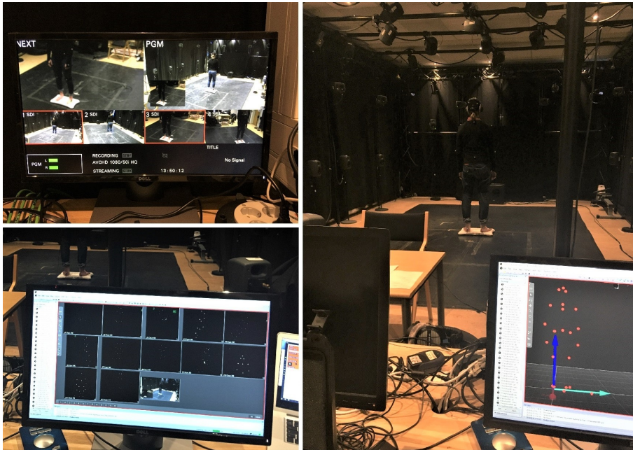
Figure 4.10: This figure displays the different ways of viewing the participant during a motion capture recording session. Upper left: Images from four regular cameras placed in the corners of the laboratory displayed using a video mixer. Bottom left: Preview of images from each of the 12 motion capture cameras as displayed in the Qualisys software. Reflections visible to the cameras are displayed as white spots on a black background. Based on such images, it is possible to ensure that cameras register only reflections from the markers (which is ideal) and not other shiny surfaces (which results in artefacts). Right: Representation of the markers, visible as red dots, in the three-dimensional space recreated in the Qualisys software from the images provided by all cameras.
