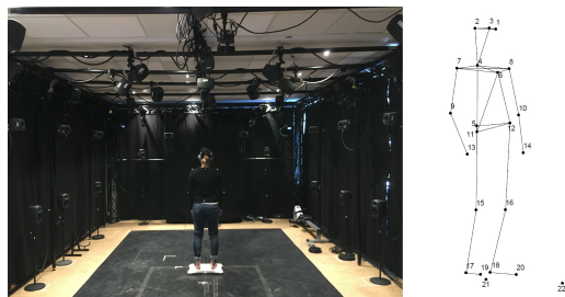
Figure 2. Left: Laboratory setup and one participant standing during the headphones condition. Written informed consent was obtained from the participant for publication of images. Right: Motion capture reconstructed markers and segments. The markers were located as follows (L, left; R, right; F, front; B, back): 1 - F head; 2 - RB head; 3 - LB head; 4 - B neck; 5 - sacrum; 6 - sternum; 7 - R shoulder; 8 - L shoulder; 9 - R elbow; 10 - L elbow; 11 - R hip; 12 - L hip; 13 - R wrist; 14 - L wrist; 15 - R knee; 16 - L knee; 17 - R heel; 18 - L heel; 19 - R toe; 20 - L toe; 21 - reference marker on the Wii board, 22 - reference marker on the floor.
