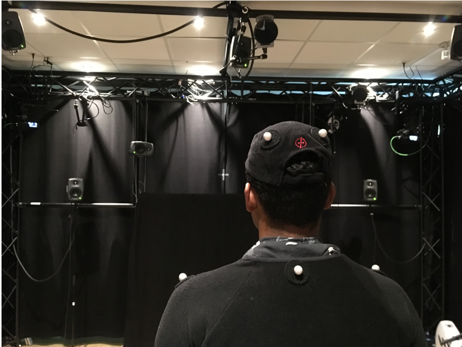
Figure 4.4: A photograph of a participant in the Headphones/Speakers experiment. Motion capture markers are attached to selected anatomical landmarks via a Velcro adhesive motion capture suit and hat. A pair of Genelec 8020 speakers (here, the pair at the level of the participants' ears) is used to present sound in the speakers listening condition. A white cross is taped to the wall (at eye level). One of the 12 motion capture cameras, facing the participant, is visible in the upper-middle section of the photo. At the level of the head markers, towards the left and right edges of the photo, there are two cameras recording audiovisual material for reference.
