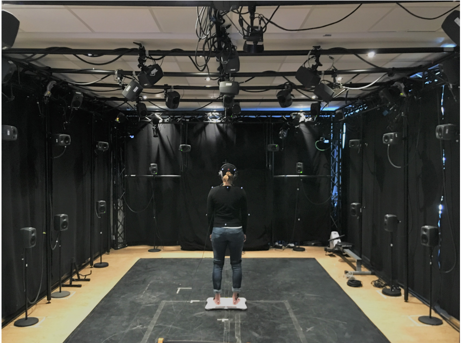
Figure 4.8: The motion capture laboratory where all the experiments took place (this is a picture from the Headphones/Speakers experiment). Several cameras and speakers are mounted on the walls, floor and ceiling. The floor is covered with a black matte material to prevent reflections from the yellow linoleum. The white tape on the floor is used for reference when placing the calibration frame on the floor (there are several configurations for different ongoing experiments in the laboratory).
