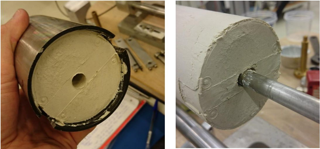
Figure 3.5 - Soil chamber (left photo) with kaolin specimen inside. The centre has been cored to fit the model pile inside (right photo).
