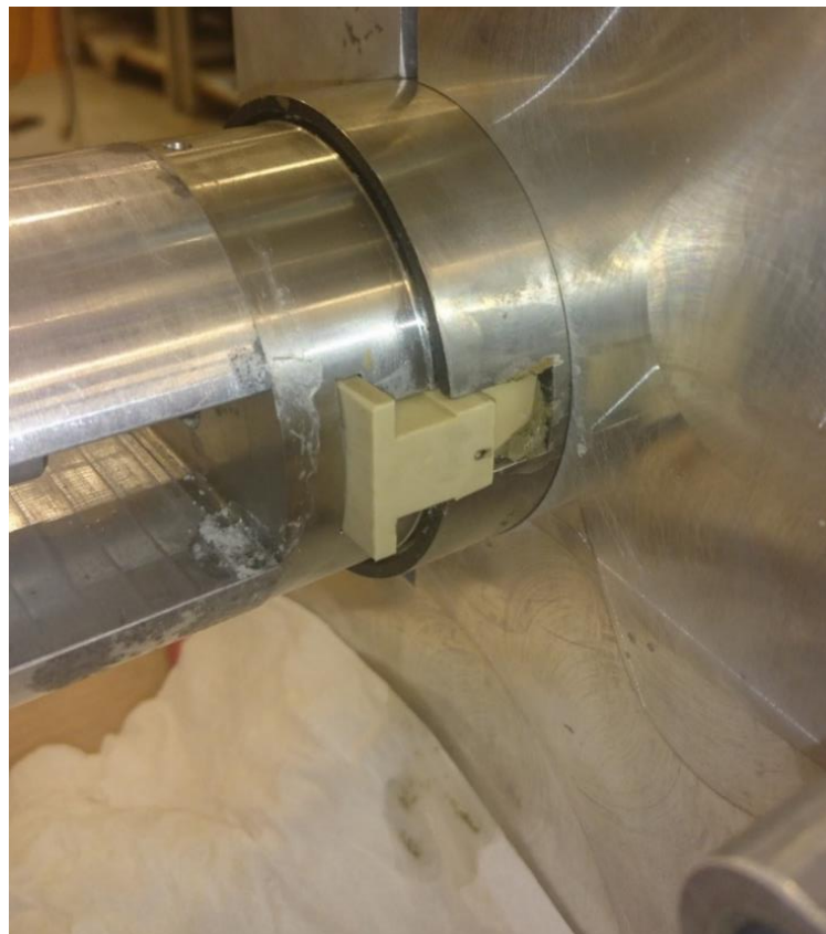
Figure 3.6 - Material squeezed out between the soil chamber and the end cap. Some wet stains on a tissue are observed below the end cap.
