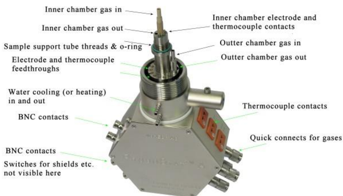
Figure 4.2 Example of a ProboStat™ measuring cell, with a description of the main component [72].
