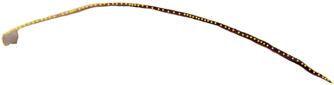
Fig. 3.1. Scanned picture of Mytilus edulis shell from Skådalen after LA-ICPMS analyses were performed. Yellow dots show each laser ablation point alongside the shell. The shell is ca. 4.5 cm in length.
