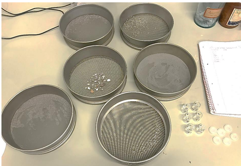
Fig. 2.9. Wet sieving of Sognsvann sample. A4 notebook for scale.
