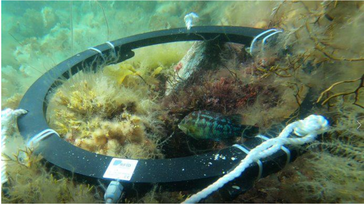
Figure 4. The underwater set up where the nest is in the middle, protected by a territorial male shown in the picture. The black circular ring is the antenna itself; every time a marked fish crosses it the detection would be registered. Photo: Maciej Karaszkiwicz.
