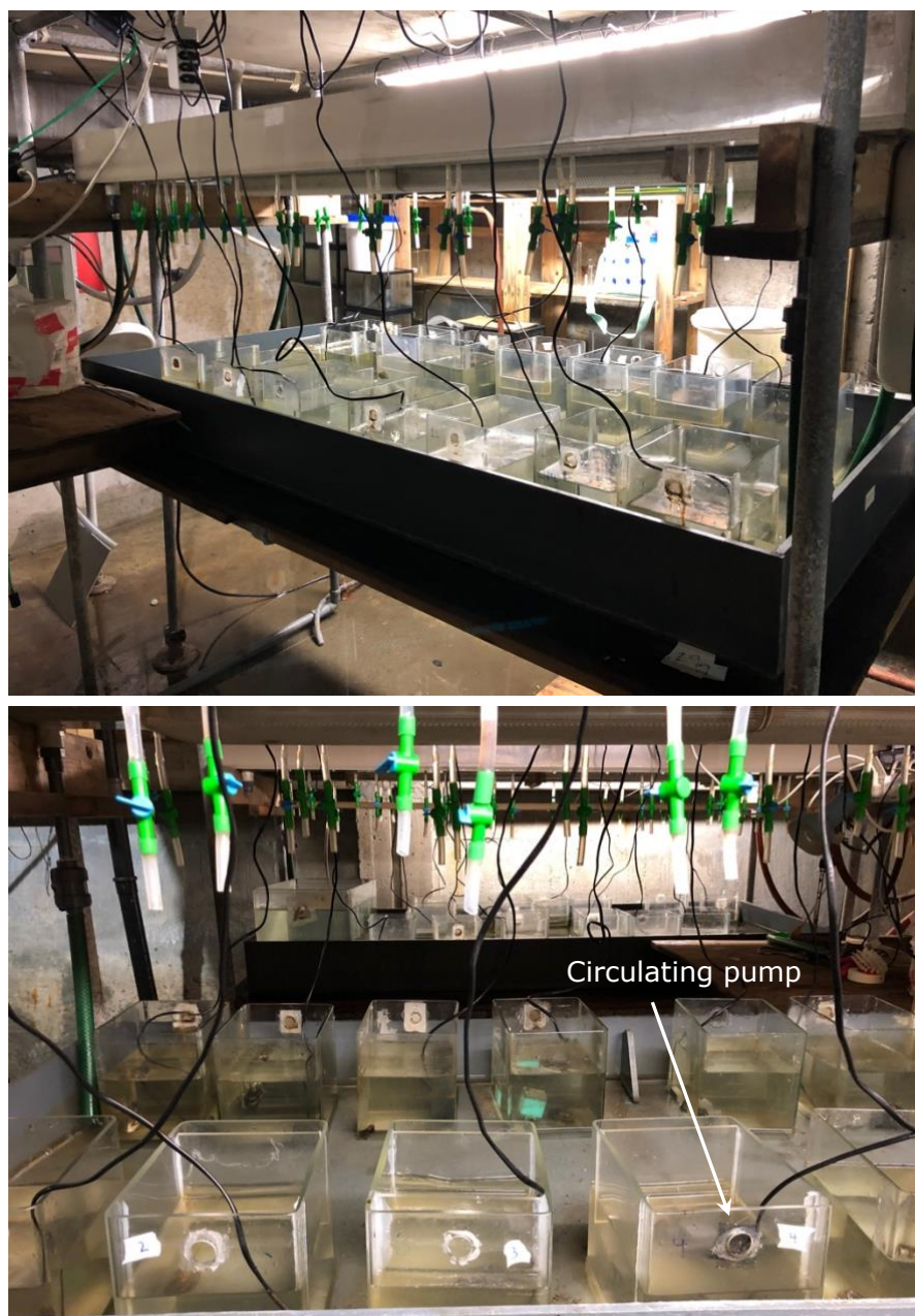
Figure 2.2. Aquaria set-up in the wetlab at NIVA Solbergstrand.
