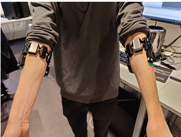
Figure 6. Placement of the EMG sensors on the arms of the guitarists. Two Delsys EMG sensors were placed on each side of the arm, right below the Myo armbands.
