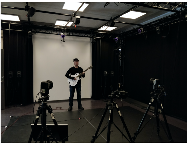
Figure 5. A participant during the recording session. Motion capture cameras can be seen hanging in the ceiling rig behind, and on stands in front of, the performer. The monitor with instructions can be seen below the front left motion capture camera.
