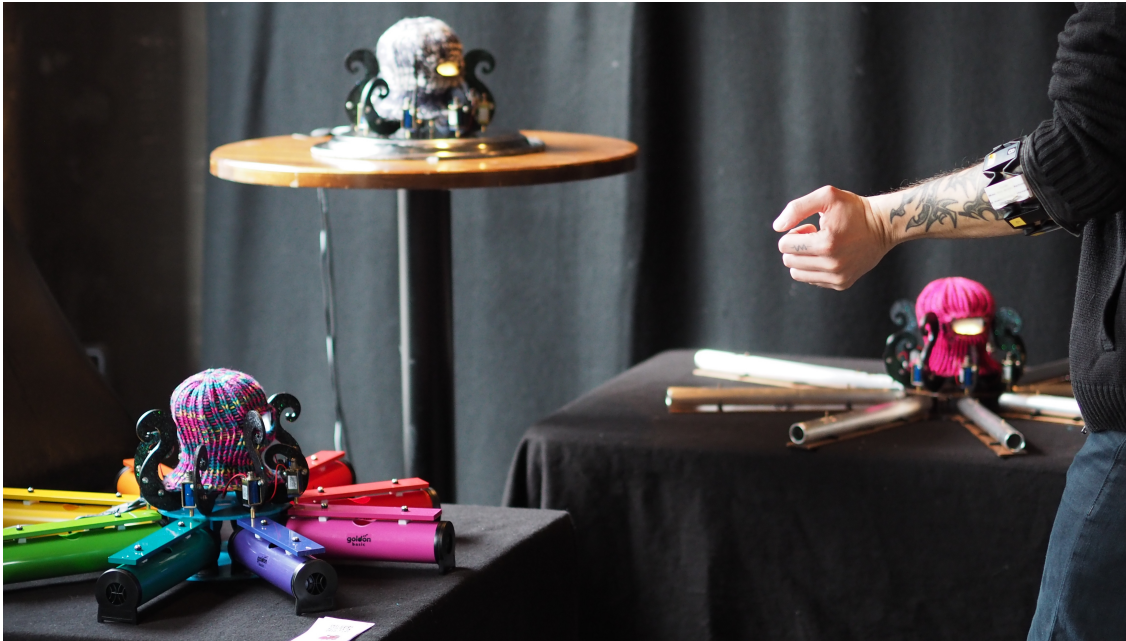
Figure 2: A human performer interacts with three Dr. Squiggles robots. Myo muscle-sensors can be seen on the arm of the human performer. The robots tap on metal rods on the table.
