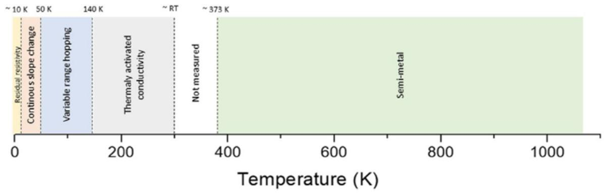
Figure 7 Temperature dependence of predominant transport mechanism under air atmosphere
