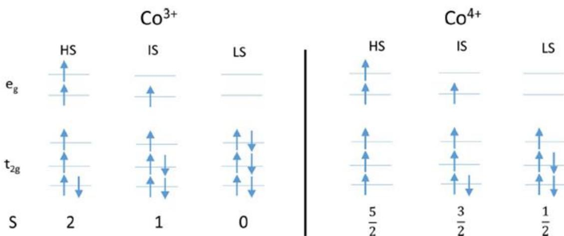
Figure 2 Possible distributions of electrons in, a high spin (HS), intermediate spin (IS) or low spin (LS) state for cobalt 3+ and 4+.
