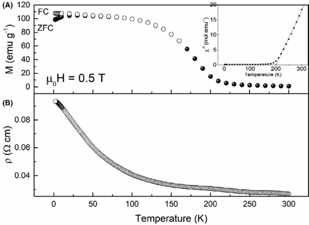
Figure 3 Magnetic susceptibility as a function of temperature under field cooling (FC) and zero-field cooling (ZFC) mode (a) and temperature dependence of resistivity (b)
