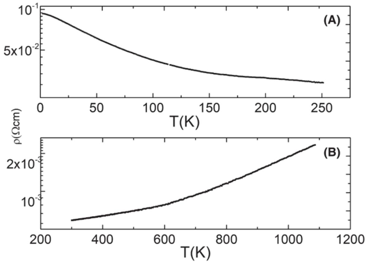
Figure 5 Temperature dependence of resistivity in air from 2 K to room temperature (a), and high temperature (b)
