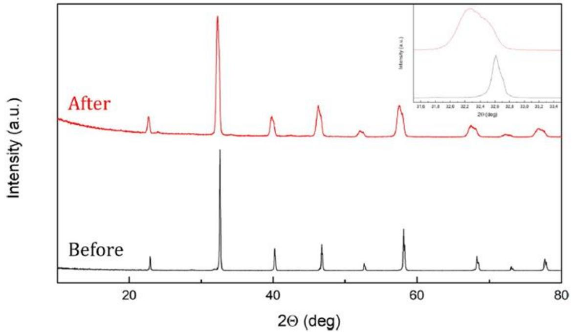
Figure 9 X-ray diffraction pattern of BLC before (black line) and after (red line) electrical measurements in Ar
