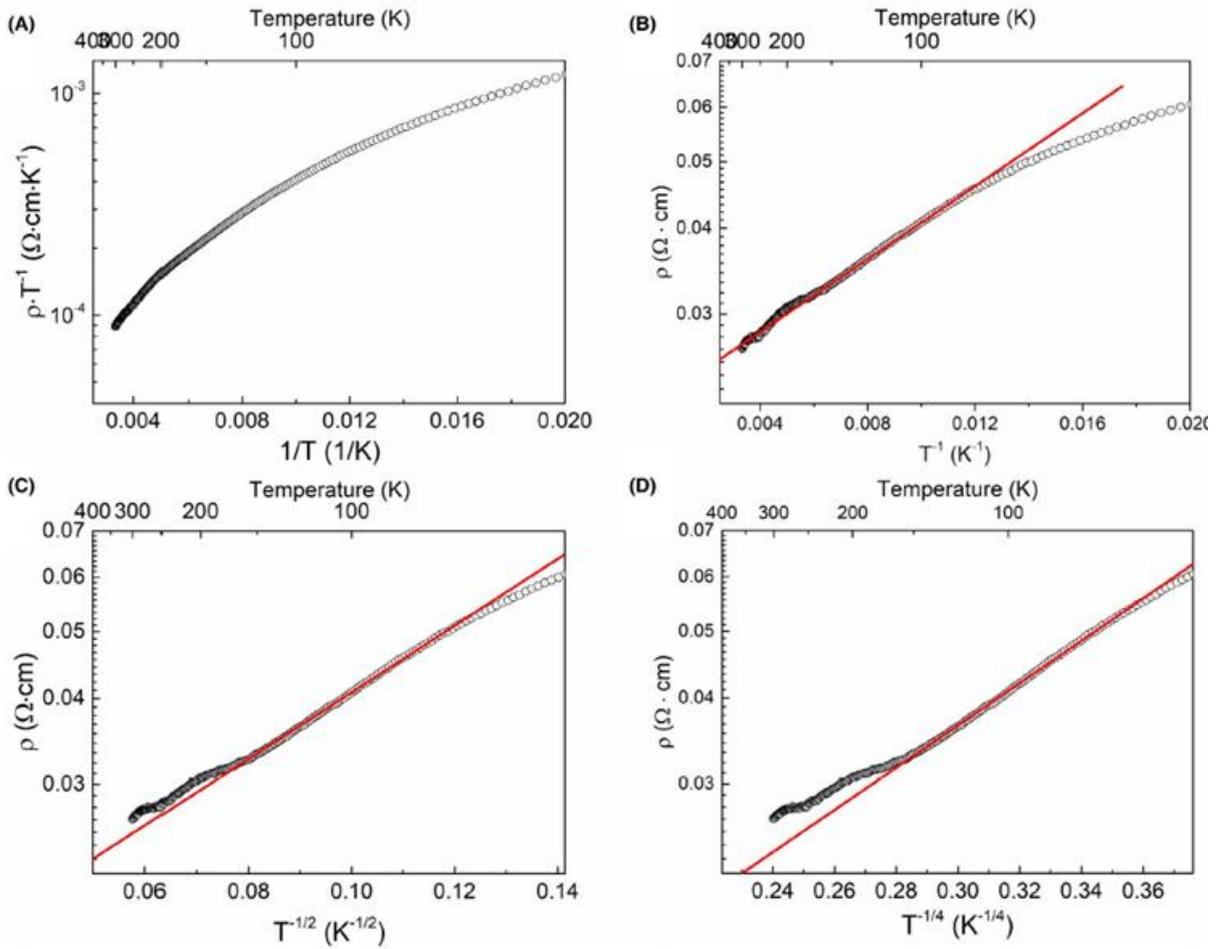
Figure 6 Low-temperature resistivity explained by the means of different transport models: small polaron hopping (a), thermally activated conductivity (b), Efros-Shklovskii mechanism (c), Variable range hopping (VRH) (d). The straight lines in red color represent the model fits and the black points are the data
