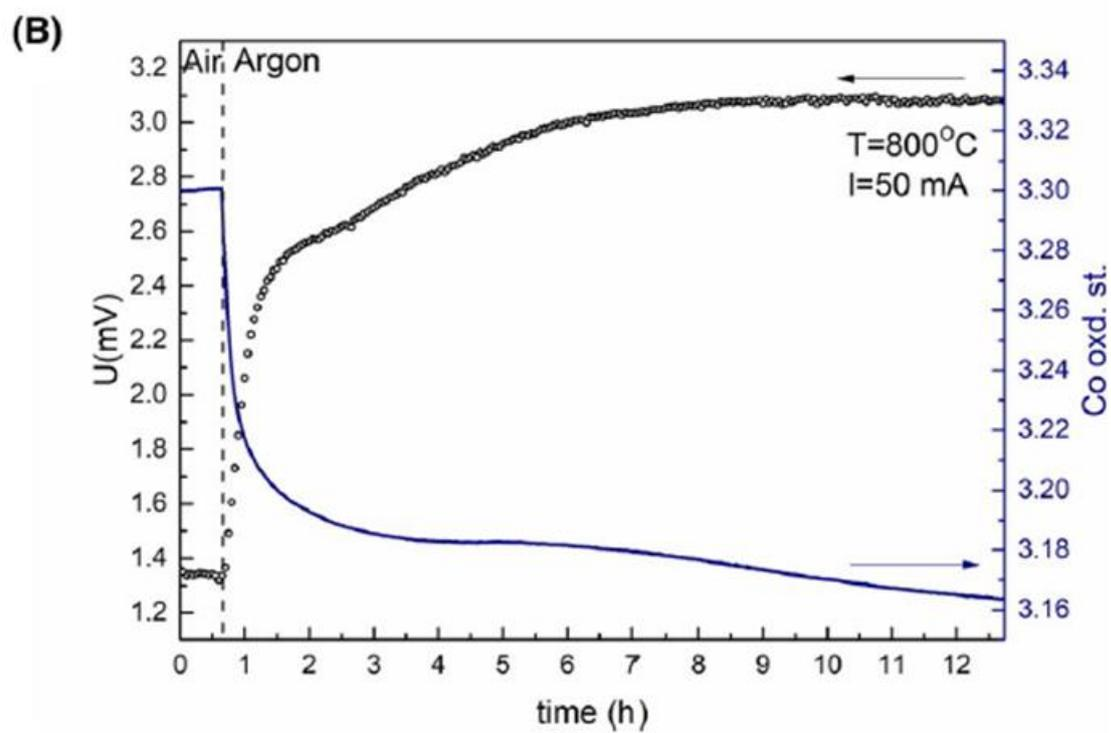
Figure 8 High-temperature resistivity in air and argon (a) and kinetics of sample reduction in argon at 800°C measured by the means of DC-4W electrical and thermogravimetric relaxation (b)
