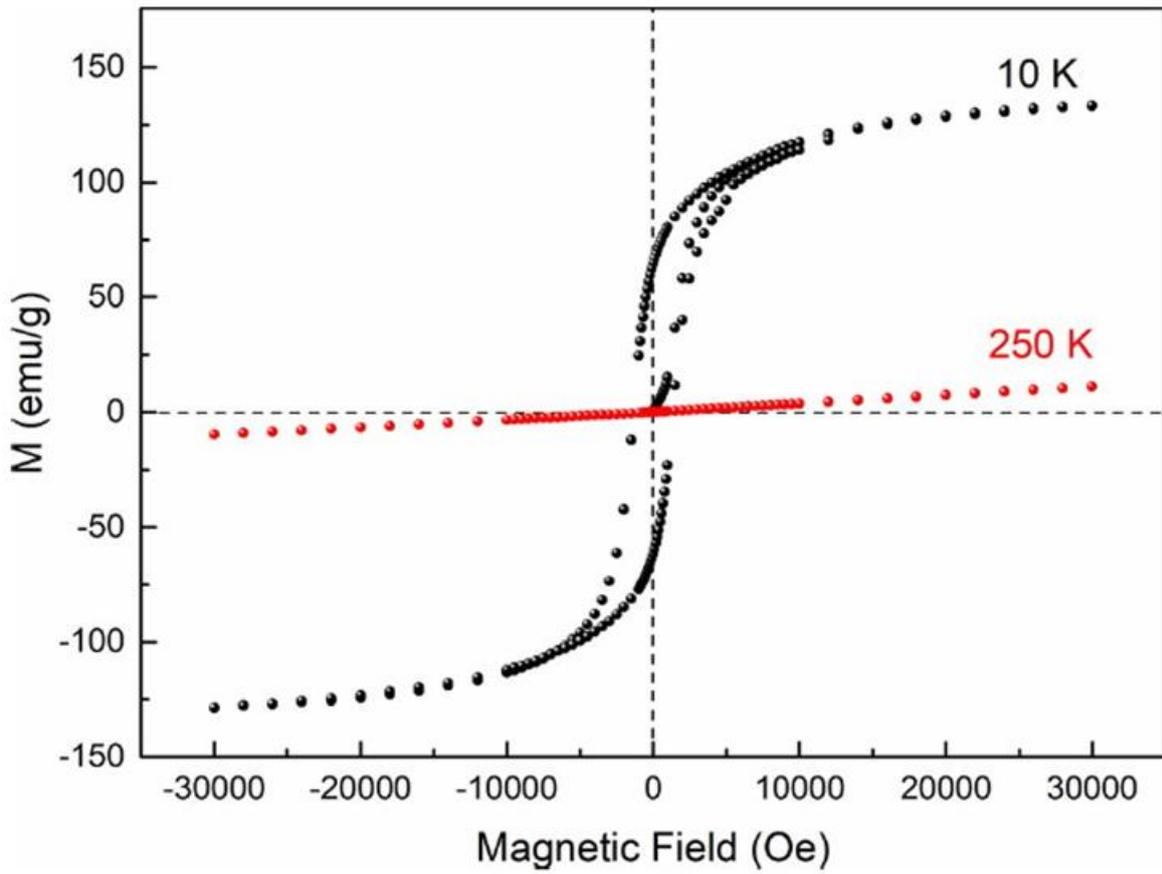
Figure 4 Field dependence of magnetization  $M(H)$  at 10 K (black) and 250 K (red)
