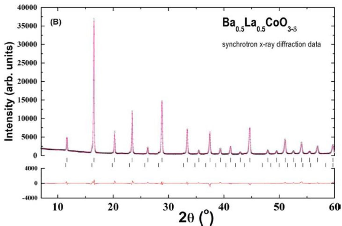
Figure 1 PND (a) SP-PXD (b) powder diffraction patterns of BLC fitted by Rietveld refinement. The wavelengths are 0.7896 Å and 1.5543 Å, respectively. Black points are experimental data, the solid profile is calculated from the refined model and the red line below is the difference plot. Vertical tick marks show Bragg peak positions.
