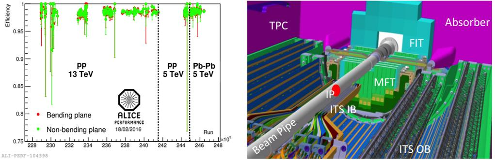
Fig. 1. The left panel shows the efficiency of the Muon Trigger Chamber RPC equipped with FEERIC, measured in ALICE in 2015. The right panel shows the position of the MFT in ALICE. The MFT half-cone is shown which is placed along the beam axis towards the Muon Spectrometer between the Interaction Point (IP) and the hadron absorber.
