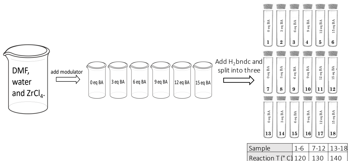
Figure 12. Schematic representation of the formation of 18 reactions for the optimization of UiO-67-bndc.
