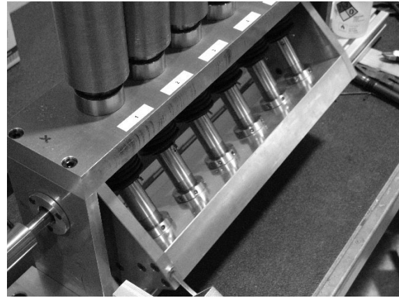
Fig. 30. The experimental set up; 6 articulations each in their own bellow and loaded with a continuous weight from above. The Jig moved as a pendulum around the axis of rotation for the joints, 45° each way. Picture courtesy of Benny Lyvén, SP technical Research Institute, Borås, Sweden
