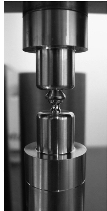
Fig. 21. On the left; the Motec thumb 6mm CrCoMo articulation used for testing. Picture courtesy of Swemac. On the right, picture of an articulation loaded in the jig. Picture courtesy of Benny Lyvén, SP technical Research Institute, Borås, Sweden
