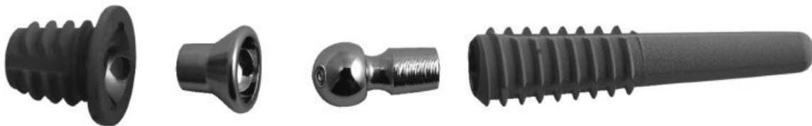
Fig. 20. Picture of the Motec® CMC1 joint replacement with its four components. The Ti_6Al_4V screw-cup had a collar and a modular CrCoMo articulation. Picture courtesy of Swemac
