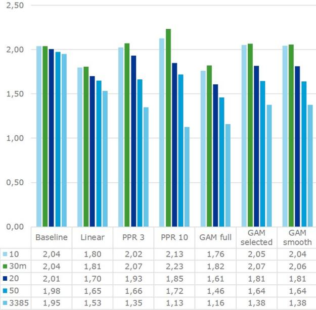
Figure 14: RMSE for the different regression methods, with  $K = 5, 10, 20, 50$  and 3385 folds. The dark blue bars, marked with 30 m, is the results of the modified 30 fold cross validation.
