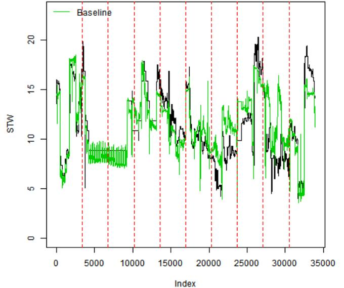
Figure 1: Prediction using the baseline method. The black line shows the observed speed through water, and the green line shows the speed through water predicted by the baseline method. The red dotted vertical lines indicates the boundary between the different folds. Here we use 10-fold cross validation.
