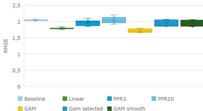
Figure 4: Boxplot of the RMSE per repetition  $l \in 1, \dots, 7$  for the different regression models, using 10-fold cross validation. For each regression method the box displays the inner quartile range, and the median is marked with a horizontal line. The mean value is indicated with a cross, while the actual values are marked with circles. The whiskers in this plot displays the maximal and minimal values.
