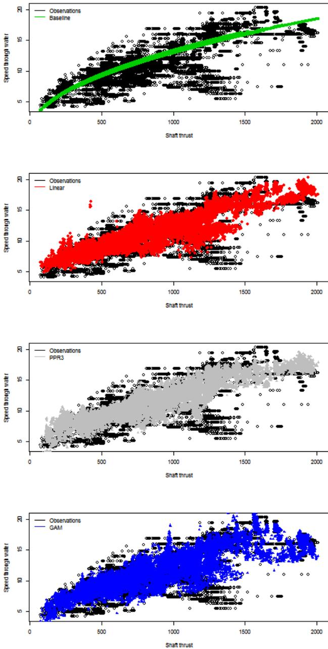
Figure 6: Scatter plot of the shaft thrust vs the speed through water and the values predicted using the different models, using 10-fold cross validation
