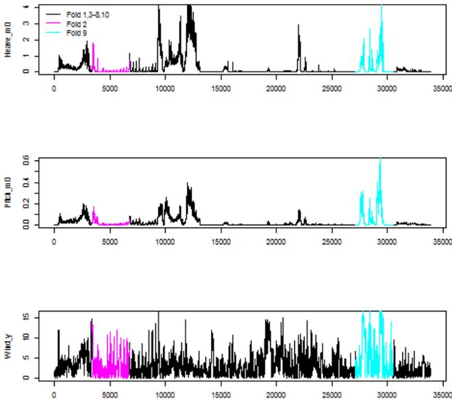
Figure 9: Traceplot of data from selected weather sensors; heave, pitch and wind perpendicular to the ship. The dataset is divided into 10 mutually exclusive folds with equal size. Fold 2 and 9 of are highlighted in magenta and cyan respectively
