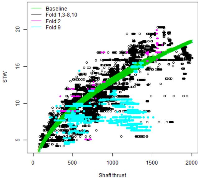
Figure 11: Scatter plot of the shaft thrust and speed through water. The green markers are the predictions based on the baseline method. The magenta and cyan markers show the observed data in fold 2 and 9 respectively. The data from the remaining folds are marked in black.
