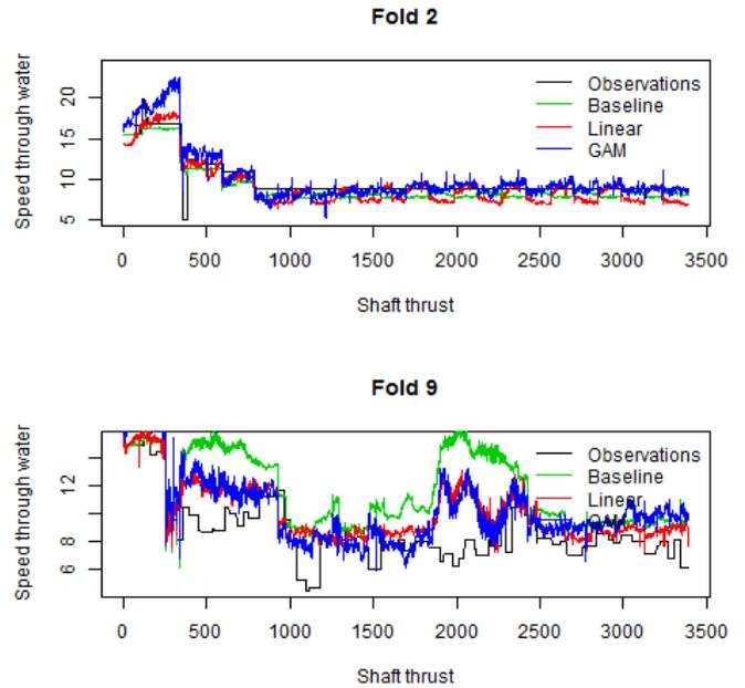
Figure 13: Prediction with different regression models on fold 2 (calm weather) and 9 (harsh weather), using 10-fold cross validation.
