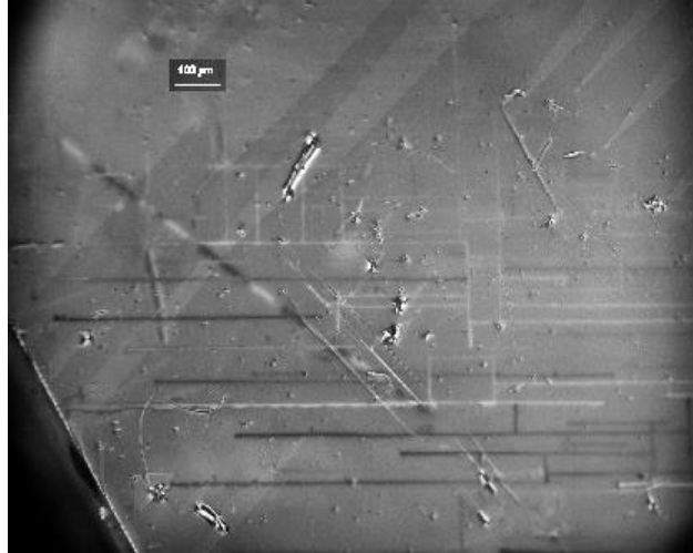
Figure 3: A stripy pattern (marked with red arrow) with periodical repetition of the fragments of positive and negative magnetic flux, on the background of weak horizontal and vertical lines, which belong to a network of nano-fractures in a superlattice with four layers of YBCO of a thickness of 750 nm. The image was recorded at 68 K after application and removal of a very small magnetic field below 1 mT.
