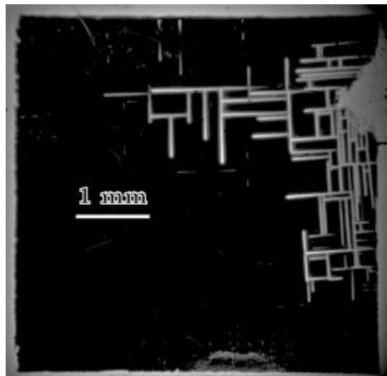
Figure 2: Magnetic flux pattern in superlattice B composed of 48 YBCO layers. The temperature of the sample at the record is 3.7 K. A magnetic field of 60 mT was applied after cooling sample in zero magnetic field.
