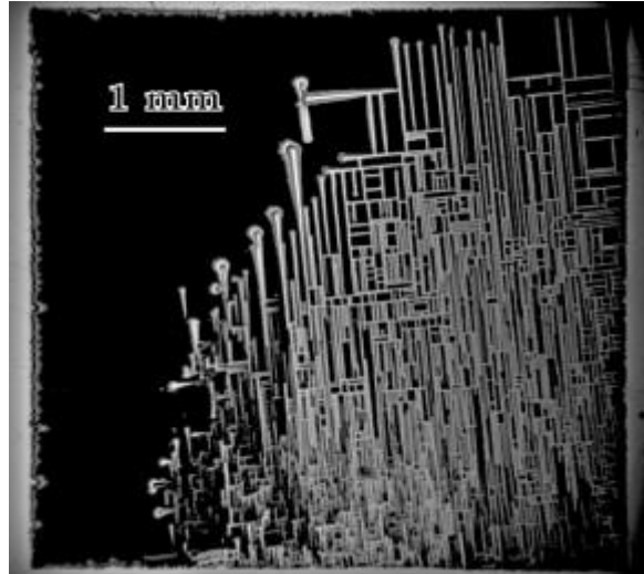
Figure 1: Magnetic flux pattern in superlattice A composed of 32 YBCO layers. The temperature of the sample is 3.7 K. A magnetic field of 60 mT was applied after cooling sample in zero magnetic field.
