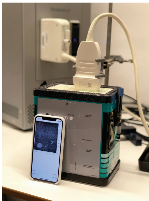
Fig. 1: The complete setup of the ultrasound probe imaging a phantom with the research scanner streaming the channel data wirelessly through the router before it is received, beamformed and displayed on the iPhone. A demo video is available at https://youtu.be/oN8cwyxGxyM .
