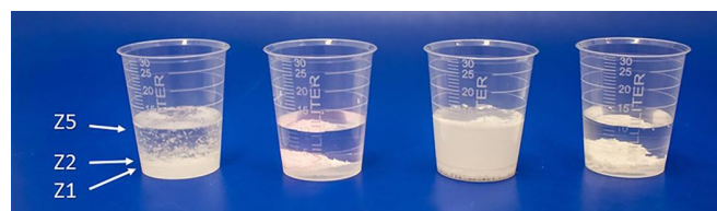
Figure 1 The four aspirin tablets upon passive dispersion in 10 mL purified water for 3 minutes. From left to right: Dispersible Aspirin (75 mg), Bayer Chewable (81 mg), Disprin (300 mg), Aspirin (500 mg). Zones 1, 2 and 5 are marked Z 1, Z 2 and Z 5, respectively.
