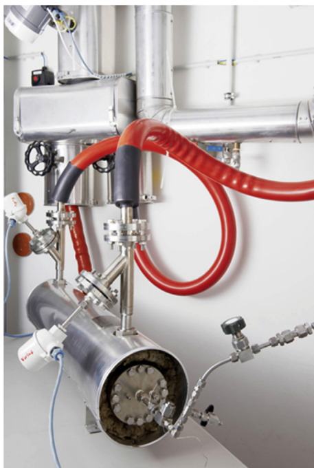
Fig. 11 – The sodium alanate-based hydrogen storage tank developed during the NESHY project showing the attachments to the testing rig.
