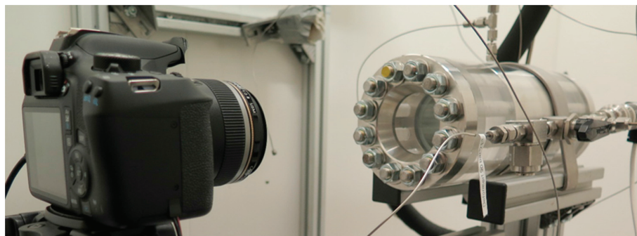
Fig. 1. Transparent autoclave with camera and injection tubing.
