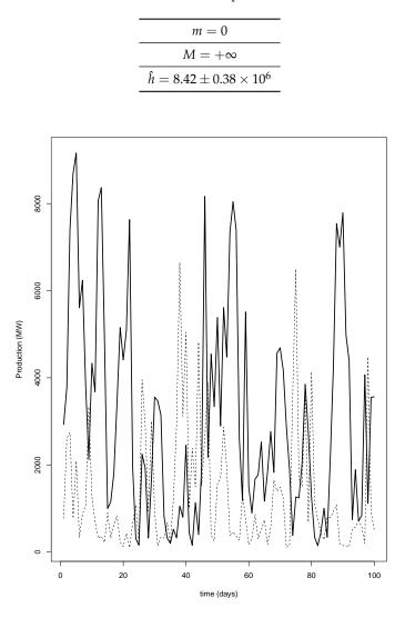
**Figure 4.** Power production time series (bold line) and power production obtained by the Betz law (dotted line), with respect to the first one hundred days.
