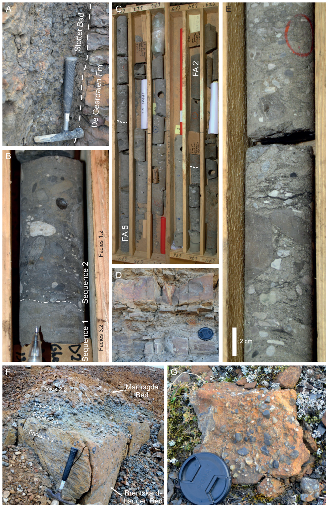
Figure 5. Examples of lag deposits (FA 1) as seen in outcrop and cores. (A) Monomictic phosphorite conglomerate (facies 1.1) at the base of the Slottet Bed at Festningen. Hammer for scale. (B) Polymictic matrix-supported conglomerate in the upper part (sequence 2) of the Wilhelmøya Subgroup in DH2. Pencil for scale. (C) FA 1 interbedded with FA 5 in the Brentskardhaugen Bed in DH4. The Brentskardhaugen Bed with sharp lower and upper boundaries towards deposits of FA 5 and FA 2, respectively. Way up from lower left to upper right. (D) Thin phosphorite conglomerate of FA 1 (above lens cap) between deposits of FA 3 below and FA 5 above in Konusdalen. Lens cap for scale. (E) Close up of (C) showing polymictic matrix-supported phosphorite conglomerates of the Brentskardhaugen Bed in DH4. The matrix is formed by fine- to medium-grained sandstones. (F) and (G) The Brentskardhaugen Bed in Konusdalen and Marhøgda. Hammer and lens cap for scale. Facies 2.2 and 2.3 of FA 2 are observed in (F) where they form part of the Marhøgda Bed.
