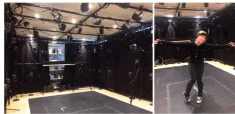
Figure 4. Lab set-up for the Experiment with 21 markers positioned on the body. 8 Motion capture cameras are hanging on the walls.
